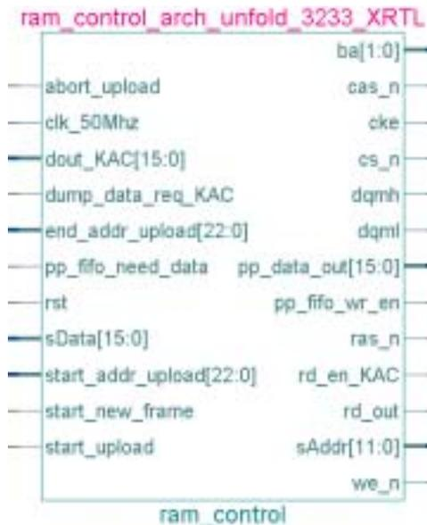
The most complex component of the design was the memory controller. It handles arbitration between different components that access the memory, interleaving read and write operations.
