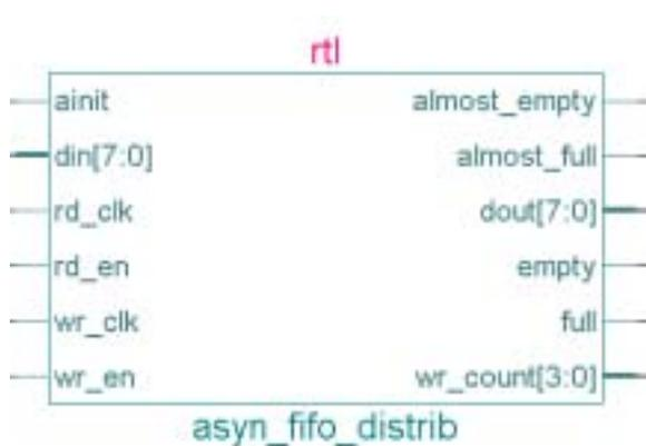
The FIFOs were produced using the Xilinx Core Generator. By using a FIFO in each component that needs access to the SDRAM, data can be buffered if RAM access is blocked by another component. Also, if SDRAM access locations are bunched together, the memory will respond faster than for accesses at addresses across bank boundaries.
