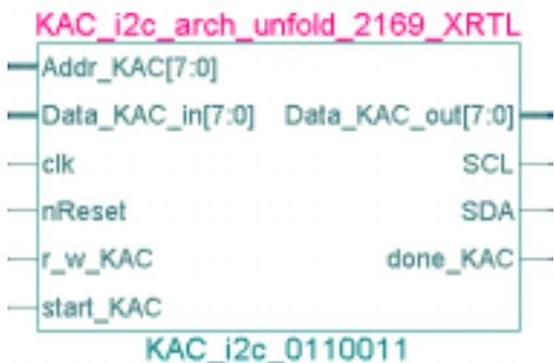
bi-directional interface. A control module was created to simplify this interface and constrain it to the specific application. Forty 8-bit control registers in the image sensor can be read and written to using a sequence of I2C events as described in section 8 of the KAC-1310 datasheet.
