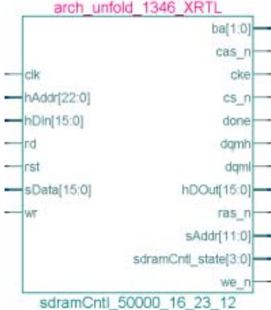
Xess has provided an SDRAM controller that makes the external 16Mx16 SDRAM look like simple SRAM. It handles refresh and bank interleaving and was available in a VHDL version. In its current state, the SDRAM controller does not support burst mode
