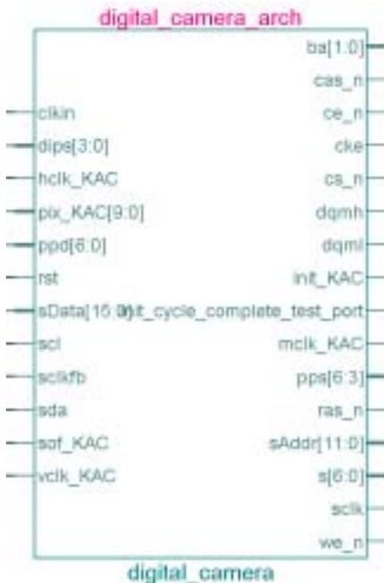
The FPGA is the main controller of the camera, handling data movement from the image sensor to the parallel port. At the top level of the camera design, ports are arranged in the following groups:
