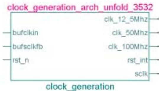
Board level deskew of the system clock was the goal of the clock generation component. This is described at <http://www.xilinx.com/products/spartan2/recipes/rec004.htm>. The principle is to sync the internal logic to the same clock that is seen by the external SDRAM, accounting for PCB and buffer delays. The clock signal is routed out of the Spartan II, then back in through a dedicated clock pin. This delay is sampled by a pair of delay lock loops which output
