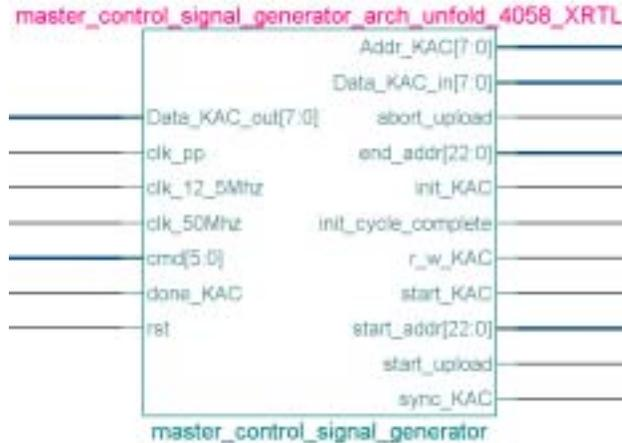
The MCSG provides status and control for top level components in the design. For instance, commands from the parallel port are decoded here, and then the control signals initiate actions in the memory controller. Startup procedures are also handled in the MCSG. The image sensor and the SDRAM require a reset and a time delay before operation can begin.
