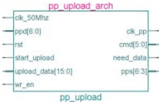
`pp_upload` component buffers data from the SDRAM in a FIFO to send through the parallel port to the image capture program on the host PC. Commands are also received and passed onto the MCSG.
