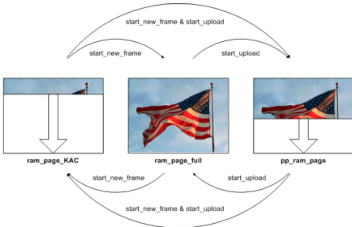
The current page is determined by the high three address bits, and there are three page registers. When a page is swapped, the page registers exchange values. The SDRAM address for a read or write is made up of the current ram page concatenated with the ram address pointer.
