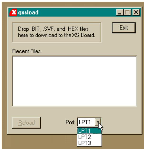
After setting the parallel port and EEPROM flag, you can download files to the XS Board simply by dragging them to the GXSLLOAD window as shown below. Once you release the mouse left-button and drop the files, GXSLLOAD will begin sending the files to the XS Board through the parallel port connection. If you drag & drop a non-downloadable file (one with a suffix other than .BIT, .SVF, or .HEX), GXSLLOAD will ignore it.
