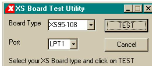
Your next step is to select the parallel port that your XS Board is connected to from the port pulldown list. GXSTEST starts with parallel port LPT1 as the default, but you can also select LPT2 or LPT3 depending upon the configuration of your PC.
