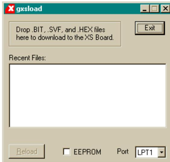
Your next step is to select the parallel port that your XS Board is connected to as shown below. GXSLLOAD starts with parallel port LPT1 as the default, but you can also select LPT2 or LPT3 depending upon the configuration of your PC. If you are programming an XS40 Board with an Atmel serial EEPROM, you can also check the EEPROM box to enable the programming of the EEPROM. In most cases, however, you will leave the box unchecked so that the FPGA or CPLD on the XS Board will be programmed.
