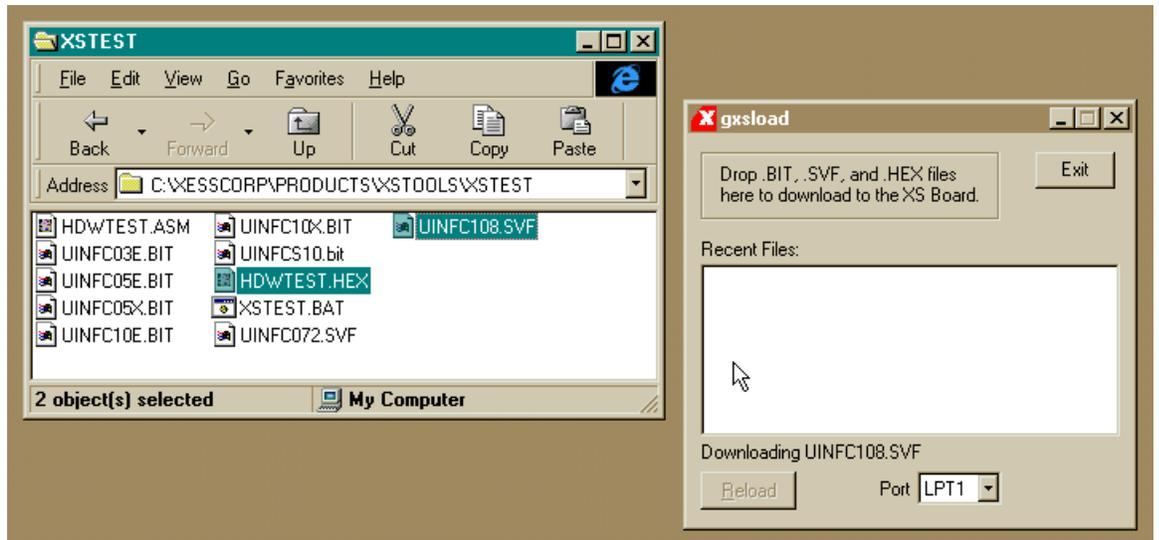
Once the downloading is finished, the file names are added to the Recent Files window and the Reload button is enabled. Now you can download these files to the XS Board just by clicking on the Reload button. This is a useful shortcut to have as you make changes to your design in Foundation and need to test the modifications.
