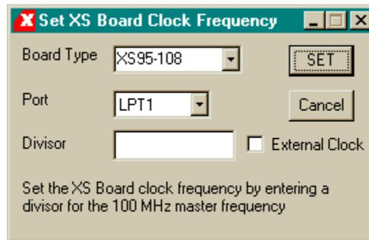
Your next step is to select the parallel port that your XS Board is connected to from the port pulldown list. GXSSETCLK starts with parallel port LPT1 as the default, but you can also select LPT2 or LPT3 depending upon the configuration of your PC. After selecting the parallel port, you select from the pulldown list the type of XS Board you have connected to the PC parallel port.
